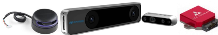
Figure [2]: Sensor images of RPLIDAR A3, Realsense T265, D435i, and VN100 from the left.
